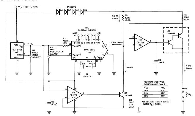
and C3 are power supply decoupling (bypass) capacitors; C4 prevents high frequency oscillations. D1 through D4 insure at least 2.5V differential between the op amp's inputs and its positive power supply under all conditions. R1 and R2 are zero scale and full scale adjustments respectively.
