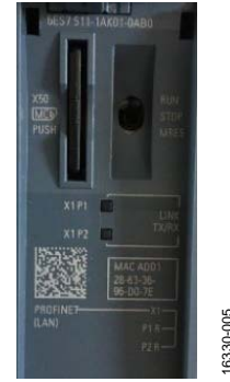
Figure 4. Siemens S7-1511 Controller MAC Address
