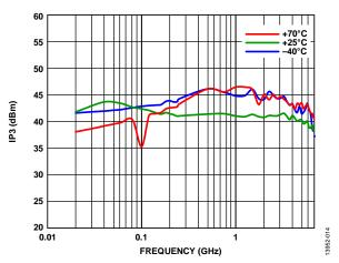
Figure 14. Output IP3 vs. Frequency
