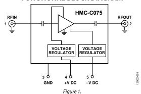
The amplifier inputs/outputs (I/Os) are dc blocked and internally matched to  $50~\Omega$ . Integrated voltage regulators allow flexible biasing of both the negative and positive supply pins, while internal bias sequencing and active bias control allows robust operation and stable performance over temperature.
