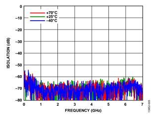
Figure 5. Isolation vs. Frequency for Various Temperatures
