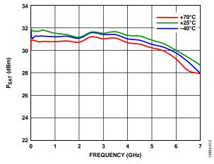
Figure 12. P<sub>SAT</sub> vs. Frequency for Various Temperatures
