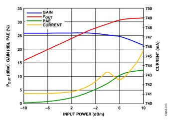
Figure 13. Output Power (Pout), Gain, and Power Added Efficiency (PAE) vs. Input Power
