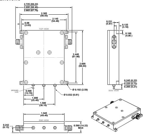
CONTROLLING DIMENSIONS ARE IN INCHES; MILLIMETER DIMENSIONS (IN PARENTHESES) ARE ROUNDED-OFF INCH EQUIVALENTS FOR REFERENCE ONLY AND ARE NOT APPROPRIATE FOR USE IN DESIGN.
