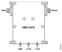
Figure 2. Pin Configuration
