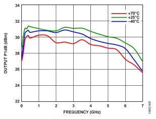
Figure 9. Output P1dB vs. Frequency for Various Temperatures
