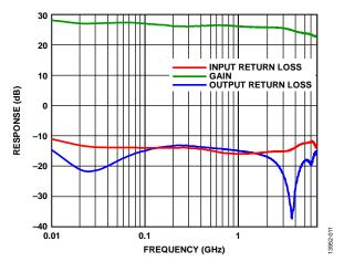
Figure 11. Gain, Input Return Loss, and Output Return Loss vs. Frequency
