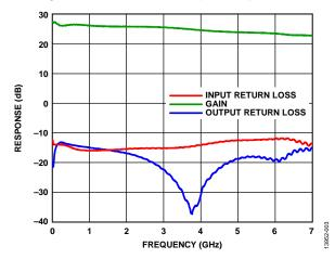
Figure 3. Gain and Input/Output Return Loss vs. Frequency
