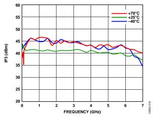
Figure 10. IP3 vs. Frequency for Various Temperatures
