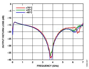
Figure 7. Output Return Loss vs. Frequency for Various Temperatures
