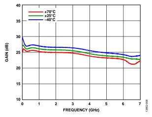
Figure 6. Gain vs. Frequency for Various Temperatures
