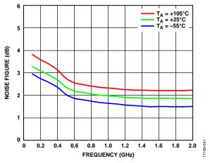
Figure 15. Noise Figure vs. Frequency at Various Temperatures, Low Frequency
