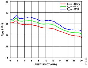
Figure 18. P<sub>SAT</sub> vs. Frequency at Various Temperatures
