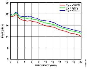
Figure 17. P1dB vs. Frequency at Various Temperatures
