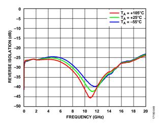
Figure 19. Reverse Isolation vs. Frequency at Various Temperatures
