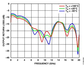
Figure 13. Output Return Loss vs. Frequency, at Various Temperatures
