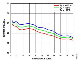
Figure 16. Output IP3 vs. Frequency at Various Temperatures
