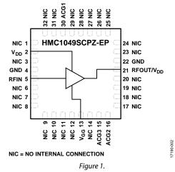
also be applied to Pin 21, although Pin 21 requires a bias tee with  $V_{DD} = 4$  V. The HMC1049SCPZ-EP amplifier input/outputs (I/Os) are internally matched to 50  $\Omega$ , and the device is supplied in a compact, leadless 5 mm × 5 mm LFCSP package.
