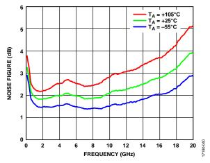
Figure 14. Noise Figure vs. Frequency at Various Temperatures
