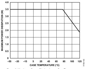
Figure 2. Maximum Power Dissipation vs. Case Temperature
