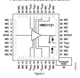
The HMC1121 exhibits excellent linearity and it is optimized for high capacity, point to point and point to multipoint radio systems. The amplifier configuration and high gain make it an excellent candidate for last stage signal amplification preceding the antenna.
