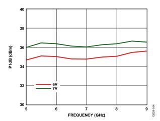
Figure 14. P1dB vs. Frequency at Various Supply Voltages
