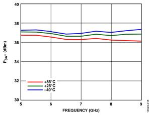
Figure 15. P<sub>SAT</sub> vs. Frequency at Various Temperatures
