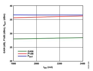
Figure 26. Gain, P1dB, and  $P_{SAT}$  vs. Supply Current ( $I_{DD}$ ) at 7 GHz
