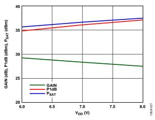
Figure 27. Gain, P1dB, and PSAT vs. Supply Voltage (VDD) at 7 GHz
