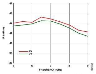
Figure 21. Output IP3 vs. Frequency at Various Supply Voltages,  $P_{OUT}/Tone = 28 \text{ dBm}$
