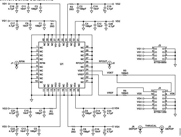
Figure 35. HMC1121 Evaluation Board Schematic
