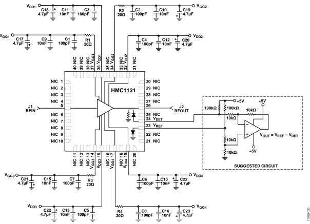
Figure 33. Typical Application Circuit
