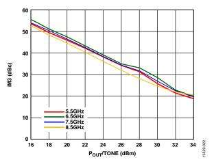
Figure 22. Output Third-Order Intermodulation (IM3) vs.  $P_{OUT}$ /Tone at  $V_{DD} = 7 V$
