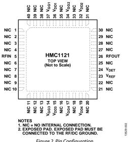
Figure 2. Pin Configuration
