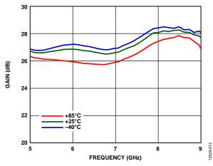
Figure 12. Gain vs. Frequency at Various Temperatures
