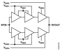
Figure 32. Simplified Block Diagram
