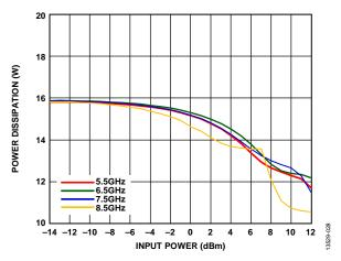
Figure 28. Power Dissipation vs. Input Power at  $T_A = 85^{\circ}C$
