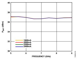
Figure 19. P<sub>SAT</sub> vs. Frequency at Various Supply Currents (I<sub>DD</sub>)
