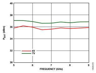
Figure 18. PSAT vs. Frequency at Various Supply Voltages
