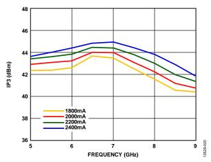
Figure 20. Output IP3 vs. Frequency at Various Supply Currents,  $P_{OUT}/Tone = 28 \text{ dBm}$
