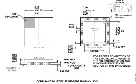
Figure 36. 40-Lead Lead Frame Chip Scale Package [LFCSP] 6 mm × 6 mm Body and 0.85 mm Package Height (HCP-40-1) Dimensions shown in millimeters
