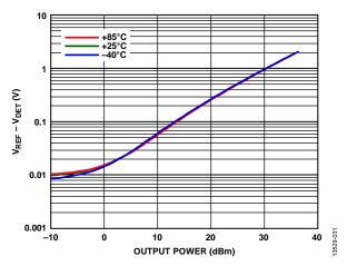
Figure 31. Detector Voltage  $(V_{REF} - V_{DET})$  vs. Output Power at Various Temperatures, at 7 GHz
