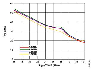
Figure 24. Output IM3 vs.  $P_{OUT}/T$ one at  $V_{DD} = 6 V$
