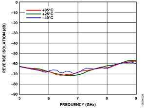
Figure 29. Reverse Isolation vs. Frequency at Various Temperatures
