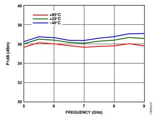
Figure 11. P1dB vs. Frequency at Various Temperatures
