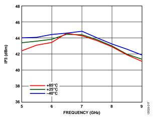
Figure 17. Output IP3 vs. Frequency at Various Temperatures,  $P_{OUT}/Tone = 28 \text{ dBm}$
