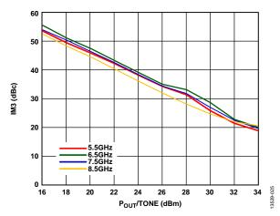
Figure 25. Output IM3 vs.  $P_{OUT}$ /Tone at  $V_{DD} = 8 V$
