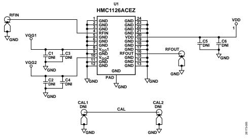
Figure 5. HMC1126-EVALZ Schematic
