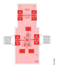
Figure 6. HMC1126-EVALZ Assembly Drawing (CAL1 and CAL2 Not Installed)
