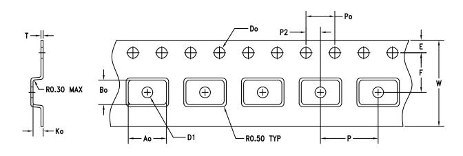
COMPONENT ORIENTATION (FORWARD TAPE AND REEL) PIN 1
