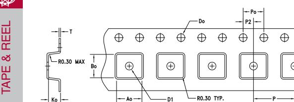
COMPONENT ORIENTATION (FORWARD TAPE AND REEL)
