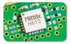
Figure 1. Model HMC613LC4B is a surfacemount SDLVA (shown mounted to a PCB) that operates from 100 MHz to 20 GHz.
