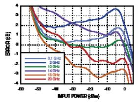
Figure 6. This plot shows gain error flatness vs. input power from 0.1 to 20 GHz for the HMC613LC4B SDLVA.
