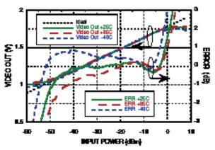
Figure 4. This plot shows the video output and log error vs. input power at 2 GHz for the HMC613LC4B SDLVA.
