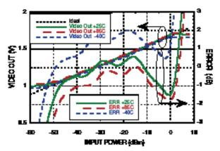
Figure 5. This plot shows the video output and log error vs. input power at 20 GHz for the HMC613LC4B SDLVA.
