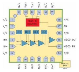
Figure 3. This block diagram shows the various functions of the HMC613LC4B SMT SDLVA.
