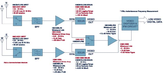
Figure 8. This block diagram for a typical RWR front end highlights the high-reliability SMT and connectorized modules (in red) from Hittite Microwave Corp
