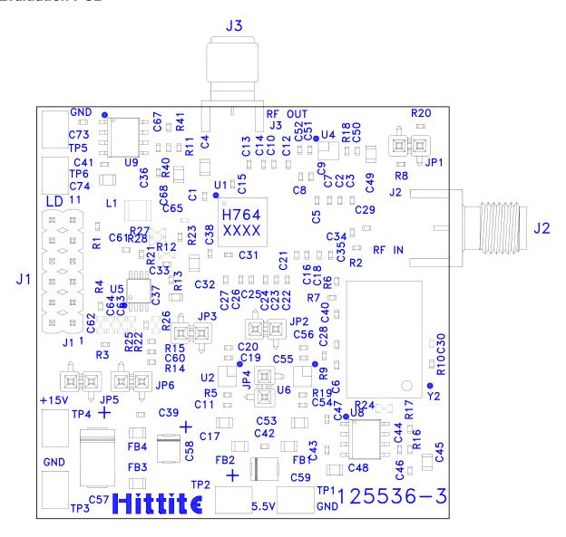
The circuit board used in the application should use RF circuit design techniques. Signal lines should have 50 Ohm impedance while the package ground leads and exposed paddle should be connected directly to the ground plane similar to that shown. A sufficient number of via holes should be used to connect the top and bottom ground planes. The evaluation circuit board shown is available from Hittite upon request.
