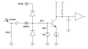
Figure 10. Reference Path Input Stage
