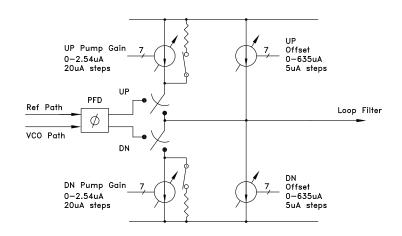
Figure 14. Charge Pump Gain and Offset Control - Reg09h
