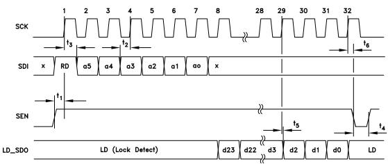
Figure 17. HMC Mode Serial Port Timing Diagram - READ
