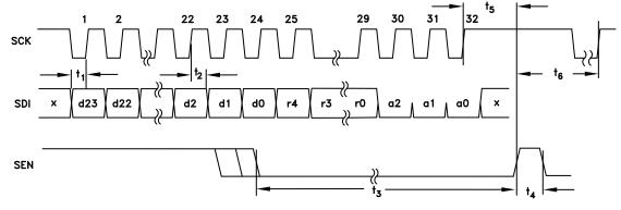
Figure 18. Open Mode - Serial Port Timing Diagram - WRITE
