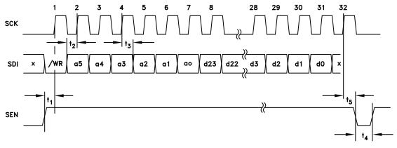
Figure 16. Serial Port Timing Diagram - HMC Mode WRITE
