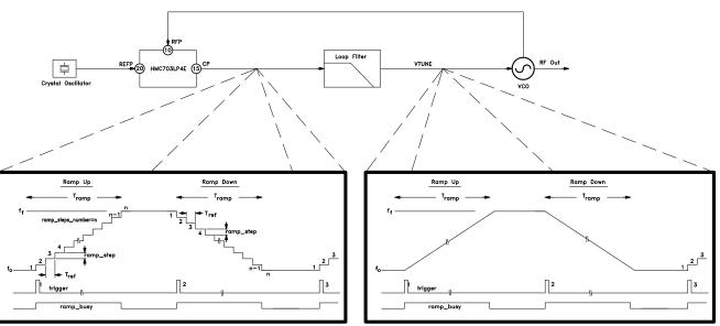
Figure 6. HMC703LP4E Sweep Function
