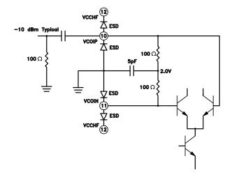
Figure 12. RF Input Stage- shown with single ended device
