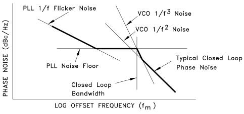
Figure 2. Figure of Merit Noise Models for the PLL
