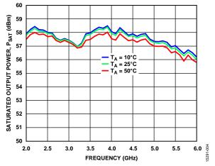
Figure 4. Saturated Output Power (P<sub>SAT</sub>) vs. Frequency at Various Temperatures
