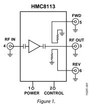
57 dBm of saturated radio frequency (RF) output power. The amplifier draws 3390 W of power from a 220 V<sub>AC</sub> supply. The RF inputs and outputs are dc blocked and matched to 50  $\Omega$  for ease of use.
