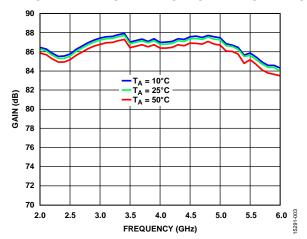
Figure 3. Gain vs. Frequency at Various Temperatures
