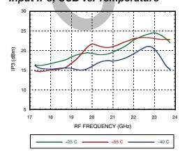
Output IP3, USB vs. Temperature
