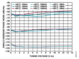
Figure 9. Single Sideband Phase Noise vs. Tuning Voltage for Various Temperatures and Frequencies
