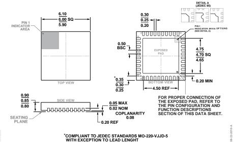
Figure 44. 40-Lead Lead Frame Chip Scale Package [LFCSP] 6 mm × 6 mm Body and 0.85 mm Package Height (HCP-40-1) Dimensions shown in millimeters
