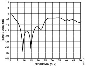
Figure 24. Return Loss vs. Frequency at  $V_{TUNE} = 6 V$
