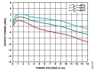
Figure 28. Output Power vs. Tuning Voltage for Various Temperatures
