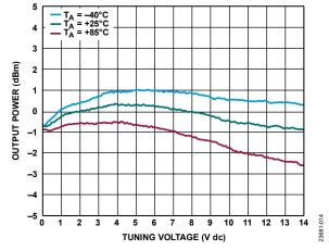
Figure 19. Ouput Power vs. Tuning Voltage for Various Temperatures
