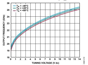
Figure 25. Output Frequency vs. Tuning Voltage for Various Temperatures
