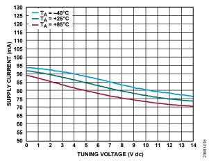
Figure 20. Supply Current vs. Tuning Voltage for Various Temperatures
