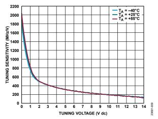
Figure 8. Tuning Sensitivity vs. Tuning Voltage for Various Temperatures
