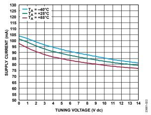
Figure 29. Supply Current vs. Tuning Voltage for Various Temperatures
