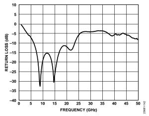
Figure 42. Return Loss vs. Frequency at  $V_{TUNE} = 6 V$
