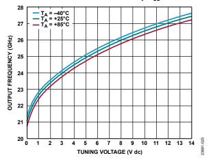
Figure 34. Output Frequency vs. Tuning Voltage for Various Temperatures
