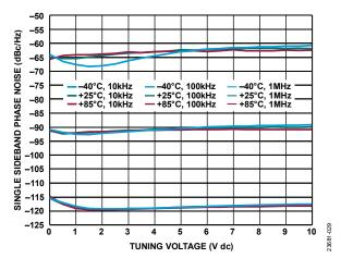
Figure 36. Single Sideband Phase Noise vs. Tuning Voltage for Various Temperatures and Frequencies (Measurement Up to 10 V Only Due to Equipment Limitation)
