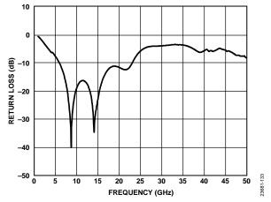
Figure 33. Return Loss vs. Frequency at  $V_{TUNE} = 6 V$
