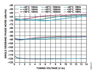
Figure 18. Single Sideband Phase Noise vs. Tuning Voltage for Various Temperatures and Frequencies
