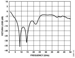
Figure 15. Return Loss vs. Frequency at  $V_{TUNE} = 6 V$
