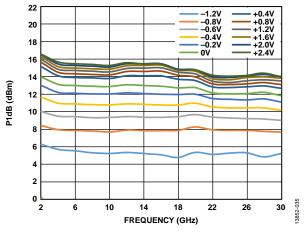
Figure 27. P1dB vs. Frequency at Various V<sub>GG</sub>2 Voltage Levels
