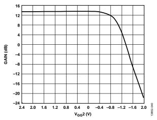
Figure 30. Gain vs. V<sub>GG</sub>2 at 10 GHz
