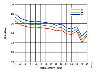
Figure 16. Output IP3 vs. Frequency at Various Supply Voltages
