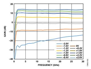
Figure 24. Gain vs. Frequency at Various V<sub>GG</sub>2 Voltage Levels
