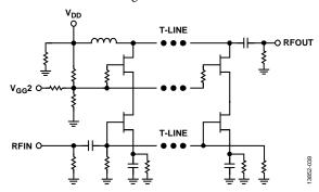
Figure 34. Architecture and Simplified Schematic
