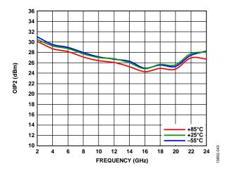
Figure 32. Output IP2 (OIP2) vs. Frequency for Various Temperatures at  $P_{\rm OUT}$  = 0 dBm/Tone
