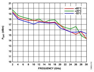
Figure 14. P<sub>SAT</sub> vs. Frequency at Various Temperatures
