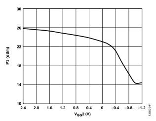
Figure 31. Output IP3 vs. V<sub>GG</sub>2 at 10 GHz
