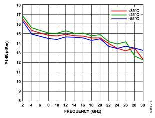
Figure 13. P1dB vs. Frequency at Various Temperatures
