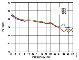
Figure 18. Output IP3 vs. Frequency for Various Temperatures at  $P_{OUT} = 0 \; dBm/Tone$
