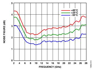
Figure 10. Noise Figure vs. Frequency at Various Temperatures
