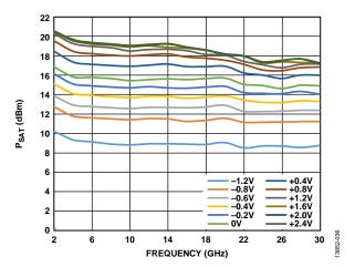
Figure 28. P<sub>SAT</sub> vs. Frequency at Various V<sub>GG</sub>2 Voltage Levels
