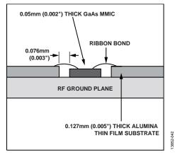
Figure 35. Routing RF Signals
