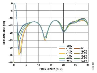
Figure 26. Output Return Loss vs. Frequency at Various  $V_{\text{GG}}$ 2 Voltage Levels
