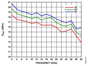
Figure 15. P<sub>SAT</sub> vs. Frequency at Various Supply Voltages
