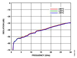
Figure 22. Reverse Isolation vs. Frequency at Various Temperatures
