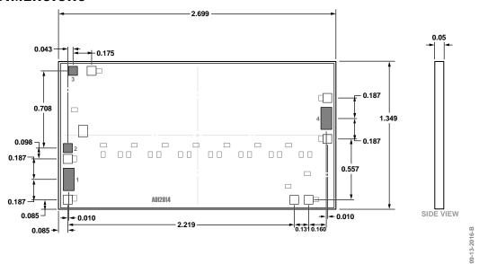
Figure 38. 4-Pad Bare Die [CHIP] (C-4-1) Dimensions shown in millimeters
