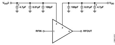
Figure 36. Typical Application Circuit
