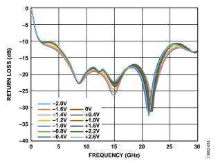
Figure 25. Input Return Loss vs. Frequency at Various V<sub>GG</sub>2 Voltage Levels
