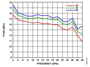
Figure 17. P1dB vs. Frequency at Various Supply Voltages
