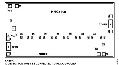
JE BOTTOM MUST BE CONNECTED TO RE/DC GROUND.
