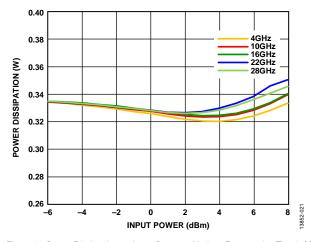
Figure 23. Power Dissipation vs. Input Power at Various Frequencies,  $T_A = 85$  °C
