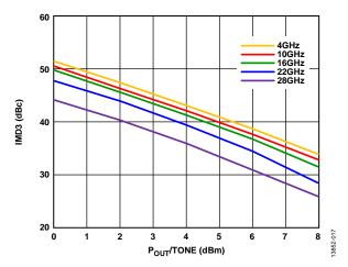
Figure 19. Output Third-Order Intermodulation (IMD3) vs.  $P_{OUT}/T$ one for Various Frequencies at  $V_{DD} = 4~V$
