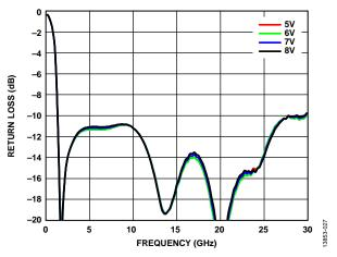
Figure 27. Output Return Loss vs. Frequency at Various Supply Voltages
