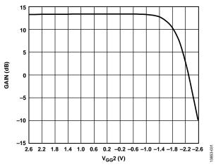
Figure 31. Gain vs. V<sub>GG</sub>2
