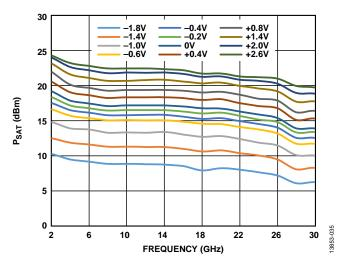
Figure 36. P<sub>SAT</sub> vs Frequency at Various V<sub>GG</sub>2 Voltages
