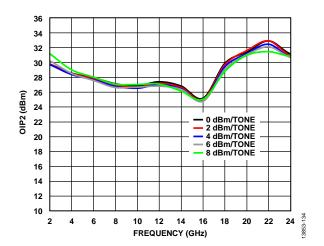
Figure 34. OIP2 vs. Frequency for Various POUT/Tone Levels
