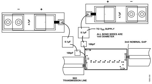
Figure 40. Assembly Diagram
