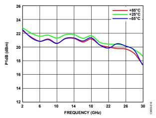
Figure 14. P1dB vs. Frequency at Various Temperatures
