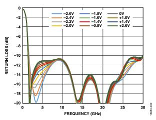
Figure 30. Output Return Loss vs. Frequency at Various V<sub>GG</sub>2 Voltages
