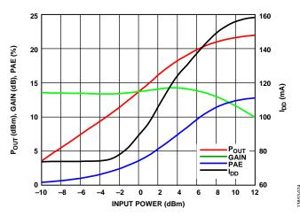
Figure 24. Power Compression at 16 GHz
