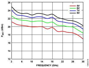
Figure 18. P<sub>SAT</sub> vs. Frequency at Various Supply Voltages
