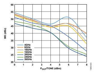
Figure 23. Output (IM3) vs.  $P_{OUT}/T$  one for Various Frequencies at  $V_{DD}=8~V$
