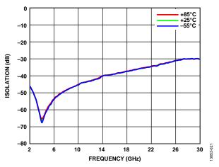
Figure 21. Reverse Isolation vs. Frequency at Various Temperatures
