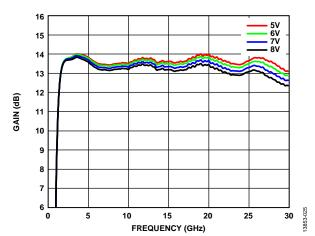
Figure 25. Gain vs. Frequency at Various Supply Voltages
