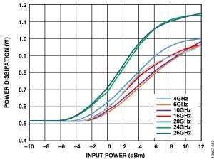
Figure 22. Power Dissipation vs. Input Power at Various Frequencies,  $T_A = 85 ^{\circ} C$
