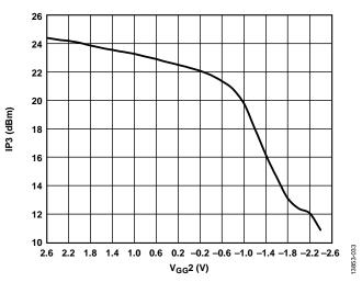
Figure 33. Output IP3 vs. V<sub>GG</sub>2 at 16 GHz
