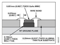
Figure 38. Routing RF Signals
