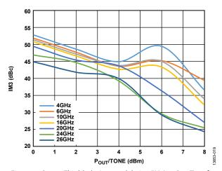
Figure 19. Output Third Order Intermodulation (IM3) vs.  $P_{OUT}$ /Tone for Various Frequencies at  $V_{DD}=6~V$
