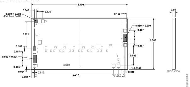
Figure 41. 4-Pad Bare Die [CHIP] (C-4-3) Dimensions shown in millimeters
