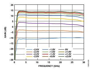
Figure 28. Gain vs. Frequency at Various V<sub>GG</sub>2 Voltages
