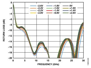
Figure 29. Input Return Loss vs. Frequency at Various V<sub>GG</sub>2 Voltages
