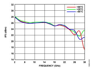
Figure 16. Output IP3 vs. Frequency for Various Temperatures at  $P_{\text{OUT}} = 0 \text{ dBm/Tone}$
