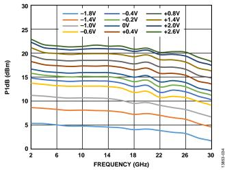
Figure 35. P1dB vs. Frequency at Various V<sub>GG</sub>2 Voltages
