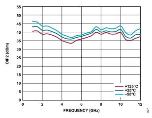
Figure 27. OIP2 vs. Frequency, 1 GHz to 12 GHz, for Various Temperatures,  $V_{DD} = 5 \text{ V}$ ,  $I_{DQ} = 55 \text{ mA}$
