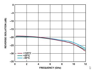
Figure 17. Reverse Isolation vs. Frequency, 200 MHz to 12 GHz, for Various Temperatures,  $V_{DD}$  = 5 V,  $I_{DQ}$  = 55 mA
