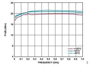
Figure 16. P1dB vs. Frequency, 0.01 GHz to 1.0 GHz, for Various Temperatures,  $V_{DD} = 5 \text{ V}$ ,  $I_{DQ} = 55 \text{ mA}$
