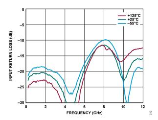
Figure 12. Input Return Loss vs. Frequency, 200 MHz to 12 GHz, for Various Temperatures,  $V_{DD}$  = 5 V,  $I_{DQ}$  = 55 mA
