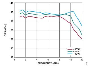
Figure 25. OIP3 vs. Frequency, 1 GHz to 12 GHz, for Various Temperatures,  $V_{DD} = 5 \text{ V}$ ,  $I_{DQ} = 55 \text{ mA}$
