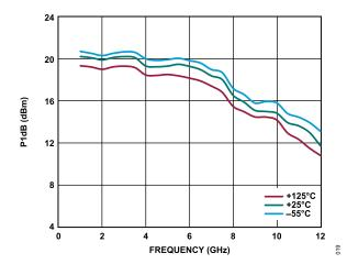
Figure 19. P1dB vs. Frequency, 1 GHz to 12 GHz, for Various Temperatures,  $V_{DD}$  = 5 V,  $I_{DQ}$  = 55 mA
