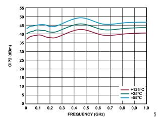
Figure 26. OIP2 vs. Frequency, 0.01 GHz to 1.0 GHz, for Various Temperatures,  $V_{DD}$  = 5 V,  $I_{DQ}$  = 55 mA
