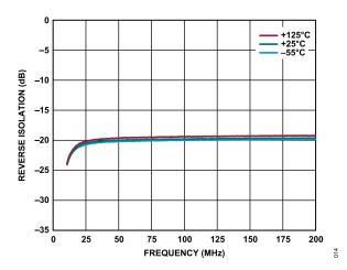
Figure 14. Reverse Isolation vs. Frequency, 10 MHz to 200 MHz, for Various Temperatures,  $V_{DD}$  = 5 V,  $I_{DQ}$  = 55 mA
