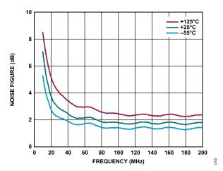
Figure 15. Noise Figure vs. Frequency, 10 MHz to 200 MHz, for Various Temperatures,  $V_{DD} = 5 \text{ V}$ ,  $I_{DQ} = 55 \text{ mA}$
