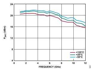
Figure 23.  $P_{SAT}$  vs. Frequency, 1 GHz to 12 GHz, for Various Temperatures,  $V_{DD}$  = 5 V,  $I_{DQ}$  = 55 mA
