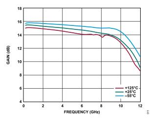
Figure 11. Gain vs. Frequency, 200 MHz to 12 GHz, for Various Temperatures,  $V_{DD}$  = 5 V,  $I_{DQ}$  = 55 mA
