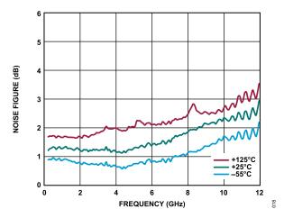
Figure 18. Noise Figure vs. Frequency, 200 MHz to 12 GHz, for Various Temperatures,  $V_{DD} = 5 \text{ V}$ ,  $I_{DQ} = 55 \text{ mA}$
