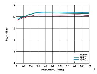
Figure 20.  $P_{SAT}$  vs. Frequency, 0.01 GHz to 1.0 GHz, for Various Temperatures,  $V_{DD}$  = 5 V,  $I_{DQ}$  = 55 mA
