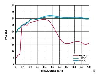
Figure 21. PAE vs. Frequency, 0.01 GHz to 1.0 GHz, for Various Temperatures,  $V_{DD} = 5 \text{ V, } I_{DQ} = 55 \text{ mA}$
