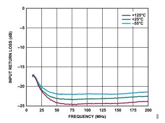
Figure 9. Input Return Loss vs. Frequency, 10 MHz to 200 MHz, for Various Temperatures,  $V_{DD}$  = 5 V,  $I_{DQ}$  = 55 mA
