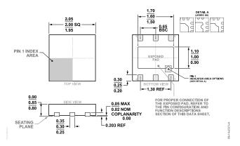
Figure 28. 6-Lead Lead Frame Chip Scale Package [LFCSP]
