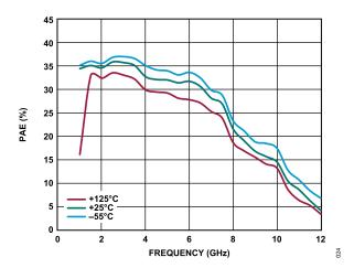
Figure 24. PAE vs. Frequency, 1 GHz to 12 GHz, for Various Temperatures,  $V_{DD}$  = 5 V,  $I_{DQ}$  = 55 mA
