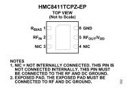
Figure 3. Pin Configuration
