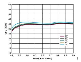
Figure 58. OIP2 vs. Frequency for Various Supply Voltages, 200 MHz to 1  ${\rm GHz}$ ,  ${\rm I}_{\rm DQ}$  = 60 mA
