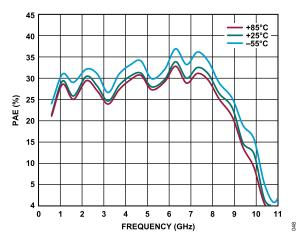
Figure 48. PAE vs. Frequency for Various Temperatures,  $V_{DD}$  = 5 V,  $I_{DQ}$  = 60 mA
