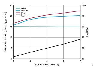
Figure 67. Gain, OP1dB,  $P_{SAT}$ , and  $I_{DQ}$  vs. Supply Voltage, Power Compression at 5 GHz,  $R_{BIAS}$  = 1.43 k $\Omega$
