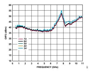
Figure 61. OIP2 vs. Frequency for Various Supply Voltages,  $I_{DQ}$  = 60 mA
