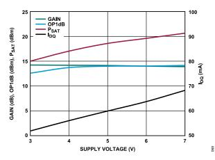
Figure 68. Gain, OP1dB,  $P_{SAT}$ , and  $I_{DQ}$  vs. Supply Voltage, Power Compression at 10 GHz,  $R_{BIAS}$  = 1.43 k $\Omega$
