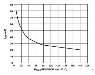
Figure 70.  $I_{DQ}$  vs.  $R_{BIAS}$  Resistor Value,  $V_{DD} = 5 \text{ V}$
