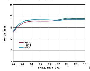
Figure 39. OP1dB vs. Frequency for Various Temperatures, 200 MHz to 1 GHz,  $V_{\rm DD}$  = 5 V,  $I_{\rm DQ}$  = 60 mA
