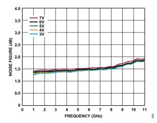
Figure 30. Noise Figure vs. Frequency for Various Supply Voltages,  $I_{DQ} = 60$
