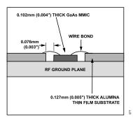
Figure 76. High Frequency Input Matching
