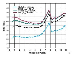
Figure 62. OIP2 vs. Frequency for Various Supply Currents,  $V_{DD} = 5 \text{ V}$
