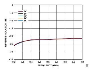
Figure 33. Reverse Isolation vs. Frequency for Various Supply Voltages, 200 MHz to 1 GHz,  $I_{DQ}$  = 60 mA
