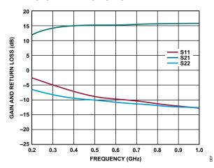
Figure 7. Gain and Return Loss vs. Frequency, 200 MHz to 1 GHz,  $V_{DD}$  = 5 V,  $I_{DQ}$  = 60 mA
