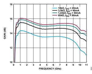
Figure 16. Gain vs. Frequency for Various Supply Currents,  $V_{DD} = 5 \text{ V}$
