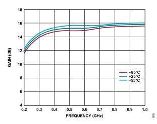
Figure 8. Gain vs. Frequency for Various Temperatures, 200 MHz to 1 GHz,  $V_{DD}$  = 5 V,  $I_{DQ}$  = 60 mA
