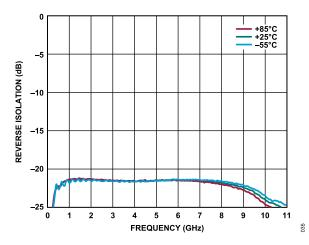
Figure 35. Reverse Isolation vs. Frequency for Various Temperatures,  $V_{DD}$  = 5 V,  $I_{DO}$  = 60 mA
