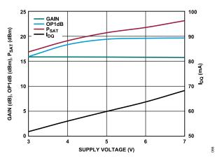
Figure 66. Gain, OP1dB,  $P_{SAT}$ , and  $I_{DQ}$  vs. Supply Voltage, Power Compression at 1 GHz,  $R_{BIAS}$  = 1.43 k $\Omega$
