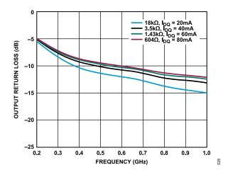
Figure 25. Output Return Loss vs. Frequency for Various Supply Currents, 200 MHz to 1 GHz,  $V_{\rm DD}$  = 5 V
