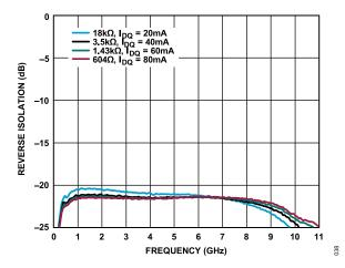
Figure 38. Reverse Isolation vs. Frequency for Various Supply Currents, V<sub>DD</sub>
