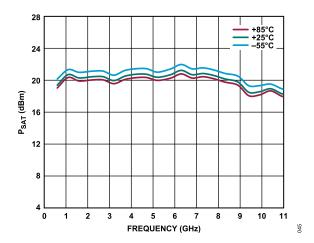
Figure 45.  $P_{SAT}$  vs. Frequency for Various Temperatures,  $V_{DD}$  = 5 V,  $I_{DQ}$  = 60 mA
