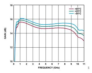
Figure 11. Gain vs. Frequency for Various Temperatures,  $V_{DD}$  = 5 V,  $I_{DQ}$  = 60 mA
