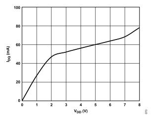
Figure 72.  $I_{DQ}$  vs.  $V_{DD}$ ,  $R_{BIAS} = 1.43 \text{ k}\Omega$
