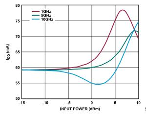
Figure 71. Drain Current ( $I_{DD}$ ) vs. Input Power for Various Frequencies,  $V_{DD}$  = 5 V,  $R_{BIAS}$  = 1.43 k $\Omega$
