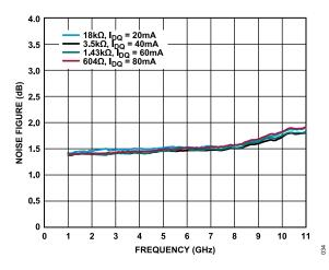
Figure 34. Noise Figure vs. Frequency for Various Supply Currents,  $V_{\rm DD}$  = 5 V
