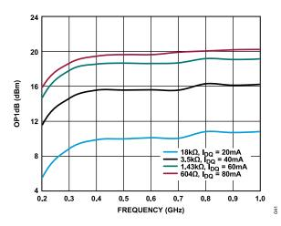
Figure 41. OP1dB vs. Frequency for Various Supply Currents, 200 MHz to 1 GHz,  $V_{DD} = 5 \text{ V}$
