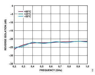
Figure 32. Reverse Isolation vs. Frequency for Various Temperatures, 200 MHz to 1 GHz,  $V_{DD}$  = 5 V,  $I_{DQ}$  = 60 mA
