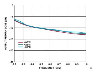
Figure 20. Output Return Loss vs. Frequency for Various Temperatures, 200 MHz to 1 GHz,  $V_{\rm DD}$  = 5 V,  $I_{\rm DQ}$  = 60 mA
