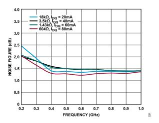
Figure 31. Noise Figure vs. Frequency for Various Supply Currents, 200 MHz to 1 GHz,  $V_{\rm DD}$  = 5 V
