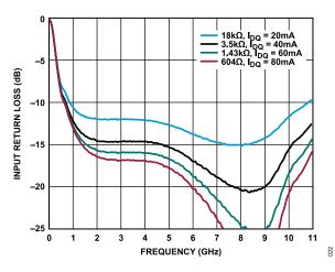
Figure 22. Input Return Loss vs. Frequency for Various Supply Currents, V<sub>DD</sub> = 5 V
