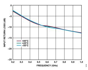
Figure 14. Input Return Loss vs. Frequency for Various Temperatures, 200 MHz to 1 GHz,  $V_{DD}$  = 5 V,  $I_{DQ}$  = 60 mA
