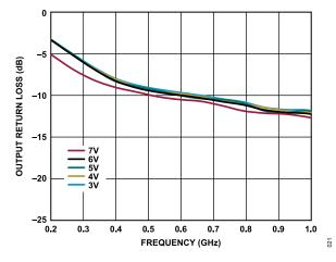
Figure 21. Output Return Loss vs. Frequency for Various Supply Voltages, 200 MHz to 1 GHz,  $I_{DQ}$  = 60 mA
