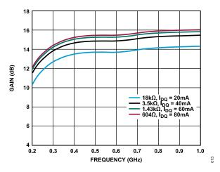
Figure 13. Gain vs. Frequency for Various Supply Currents, 200 MHz to 1 GHz,  $V_{DD}$  = 5 V
