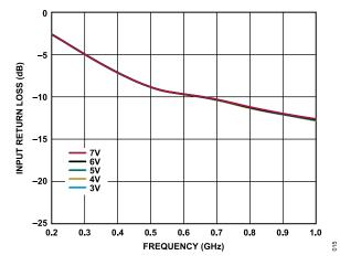
Figure 15. Input Return Loss vs. Frequency for Various Supply Voltages, 200 MHz to 1 GHz,  $I_{DQ}$  = 60 mA
