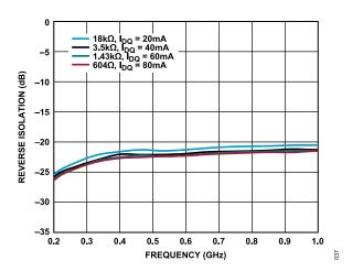
Figure 37. Reverse Isolation vs. Frequency for Various Supply Currents, 200 MHz to 1 GHz,  $V_{\rm DD}$  = 5 V
