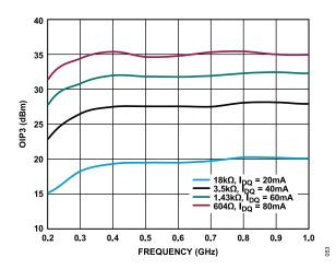
Figure 53. OIP3 vs. Frequency for Various Supply Currents, 200 MHz to 1 GHz,  $V_{DD}$  = 5 V
