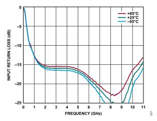
Figure 17. Input Return Loss vs. Frequency for Various Temperatures,  $V_{DD}$  = 5 V,  $I_{DO}$  = 60 mA
