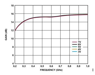
Figure 9. Gain vs. Frequency for Various Supply Voltages, 200 MHz to 1 GHz,  $I_{DQ}$  = 60 mA
