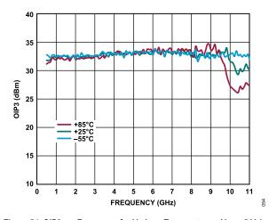
Figure 54. OIP3 vs. Frequency for Various Temperatures,  $V_{DD}$  = 5 V,  $I_{DQ}$  = 60 mA,  $P_{OUT}$  = 0 dBm per Tone
