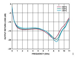
Figure 23. Output Return Loss vs. Frequency for Various Temperatures,  $V_{DD}$ = 5 V,  $I_{DQ}$  = 60 mA
