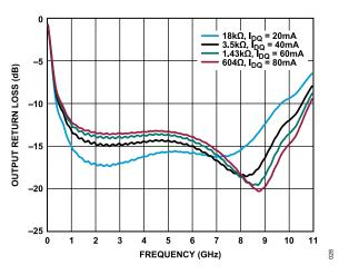
Figure 28. Output Return Loss vs. Frequency for Various Supply Currents,  $V_{DD}$  = 5 V
