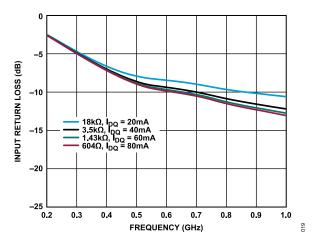
Figure 19. Input Return Loss vs. Frequency for Various Supply Currents, 200 MHz to 1 GHz,  $V_{\rm DD}$  = 5 V
