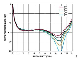
Figure 24. Output Return Loss vs. Frequency for Various Supply Voltages,  $I_{DO}$  = 60 mA
