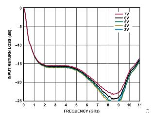
Figure 18. Input Return Loss vs. Frequency for Various Supply Voltages, I<sub>DQ</sub> = 60 mA
