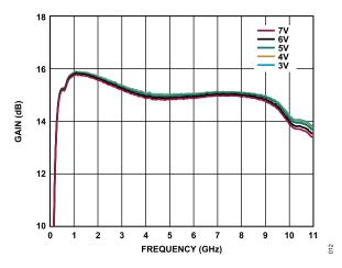
Figure 12. Gain vs. Frequency for Various Supply Voltages,  $I_{DQ} = 60 \text{ mA}$
