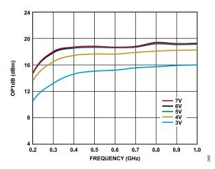
Figure 40. OP1dB vs. Frequency for Various Supply Voltages, 200 MHz to 1 GHz,  $I_{DQ}$  = 60 mA
