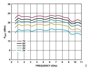
Figure 46.  $P_{SAT}$  vs. Frequency for Various Supply Voltages,  $I_{DQ}$  = 60 mA
