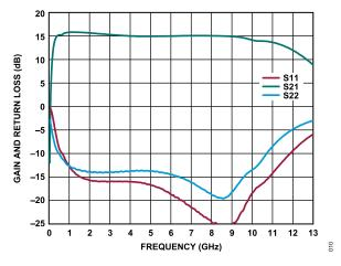
Figure 10. Gain and Return Loss vs. Frequency,  $V_{DD}$  = 5 V,  $I_{DQ}$  = 60 mA
