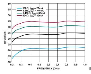
Figure 59. OIP2 vs. Frequency for Various Supply Currents, 200 MHz to 1 GHz,  $V_{\rm DD}$  = 5 V
