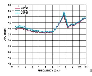
Figure 60. OIP2 vs. Frequency for Various Temperatures,  $V_{DD}$  = 5 V,  $I_{DQ}$  = 60 mA,  $P_{OUT}$  = 0 dBm per Tone
