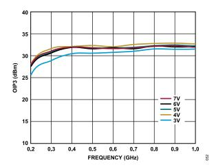
Figure 52. OIP3 vs. Frequency for Various Supply Voltages, 200 MHz to 1  $\,$  GHz,  $I_{\rm DQ}$  = 60 mA
