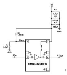
Figure 74. Typical Application Circuit
