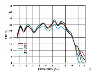
Figure 49. PAE vs. Frequency at Various Supply Voltages,  $I_{DQ}$  = 60 mA
