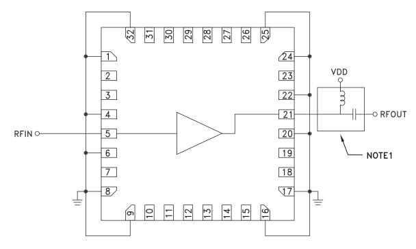
NOTE 1: Drain Bias (Vdd) must be applied through a broadband bias tee or external bias network.
