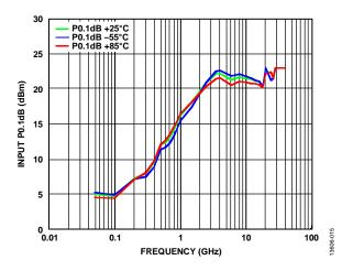
Figure 14. Input P0.1dB vs. Low Frequency over Temperature,  $V_{CTL} = -3 V$
