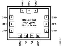
Figure 3. Pin Configuration
