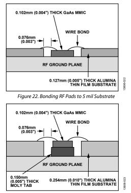
Figure 23. Bonding RF Pads to 10 mil Substrate
