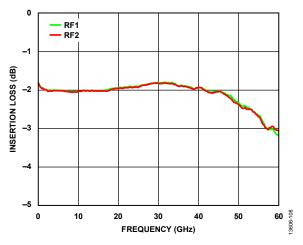
Figure 8. Insertion Loss Between RFC and RF1/RF2 vs. Frequency
