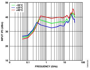
Figure 21 Input IP3 vs. Low Frequency over Temperature,  $V_{CTL} = -3 V$
