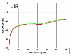
Figure 7. Isolation Between RFC and RF1/RF2 vs. Frequency
