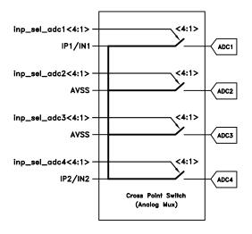
Figure 8: ADC input signals through Cross Point Switch
