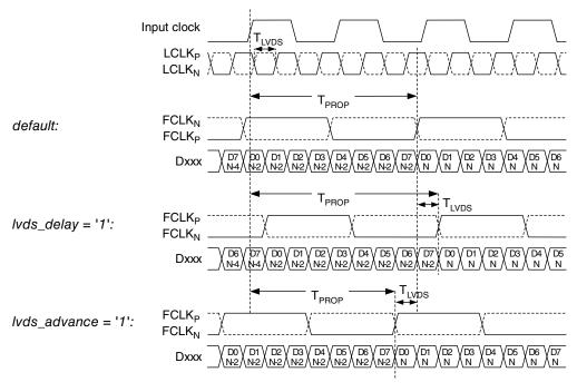
Figure 9: LVDS output timing adjustment
