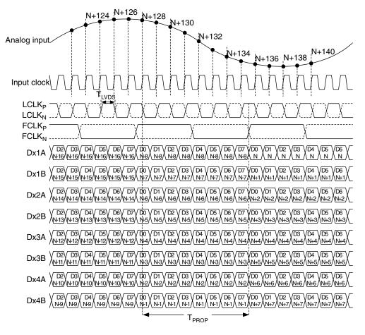
Figure 5: Single channel - LVDS timing 8-bit output
