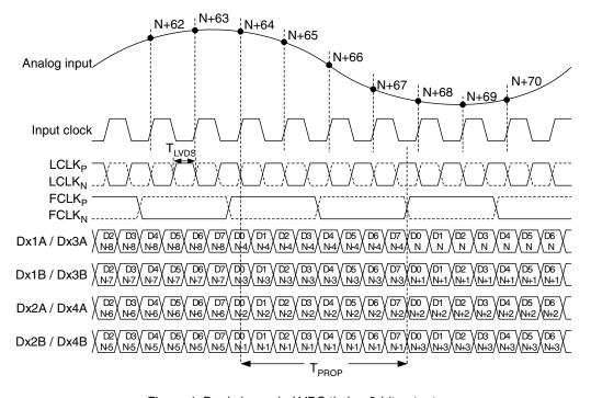
Figure 4: Dual channel - LVDS timing 8-bit output
