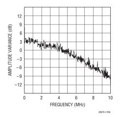
Figure 4. RMS Amplitude Holds Within ±2dB Before Sagging Beyond 5MHz
