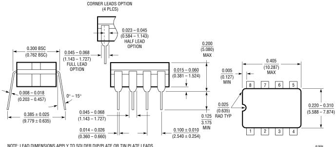
NOTE: LEAD DIMENSIONS APPLY TO SOLDER DIP/PLATE OR TIN PLATE LEADS.
