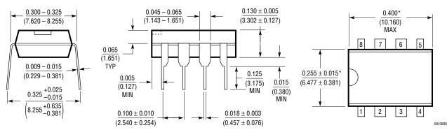
\*THESE DIMENSIONS DO NOT INCLUDE MOLD FLASH OR PROTRUSIONS. MOLD FLASH OR PROTRUSIONS SHALL NOT EXCEED 0.010 INCH (0.254mm)
