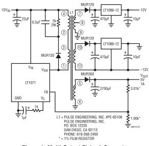
Figure 1. Multi-Output Flyback Converter
