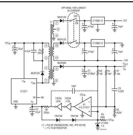
Figure 3. Multi-Output, Transformer Coupled Low Quiescent Current Converter
