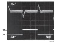
Figure 3. Upper Trace: 5V Output, Transient Load Response (50mV/DIV) Bottom Trace: Load Current (1A/DIV)
