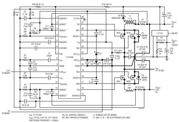
Figure 2. Two Square Inch 5V/3.3V/12V Portable Power Supply
