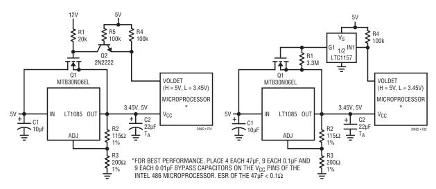
Figure 1. Bypass Circuit for 3.xxV and 5V Microprocessor Swaps Using Transistor Buffer
