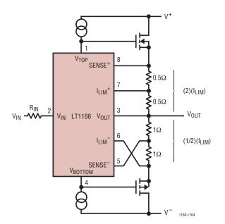
Figure 4. Tapping Current Limit Resistors
