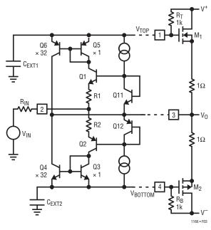
Figure 3. Input Stage Driving Gates
