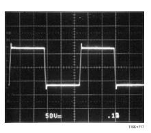
Figure 17. 2kHz Square-Wave,  $C_L = 1\mu F$
