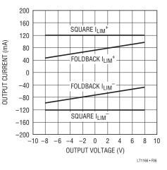
Figure 6. Output Current vs Output Voltage
