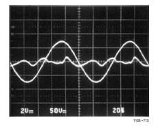
Figure 15. 0.3% THD at 10kHz,  $P_0$  = 350W,  $R_L$  = 8 $\Omega$
