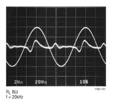
Figure 21. 100W 20kHz Sine Wave and Its Distortion
