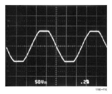
Figure 16. Clipping at 1kHz,  $R_L = 8\Omega$
