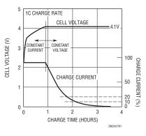
Figure 1. Typical Lithium-Ion Charge Characteristics
