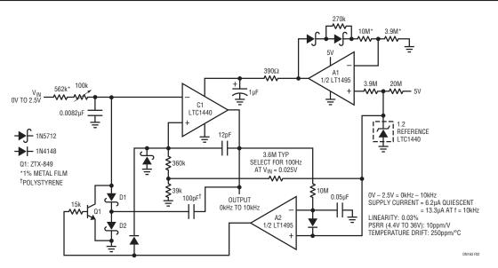
Figure 2. OkHz to 10kHz Voltage to Frequency Converter Consumes Only 13µA
