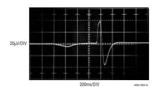
Figure B4. A Ceramic Capacitor Responds to Light Pencil Tapping. Piezoelectric Based Response Approaches  $80\mu V_{P\text{-}P}$
