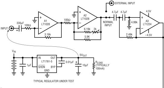
ALL RESISTORS 1% METAL FILM  $4.7\mu F \text{ CAPACITORS} = \text{MYLAR}, \text{WIMA MKS-2} \\ 330\mu F \text{ CAPACITORS} = \text{SANYO OSCON} \\ \pm 4.5\text{V DERIVED FROM 6AA CELLS} \\ \text{POWER REGULATOR FROM APPROPRIATE} \\ \text{NUMBER OF D SIZE BATTERIES}$
