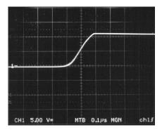
Figure 5. Switch Rise Time at Light Loads
