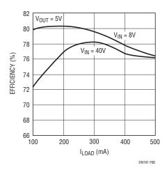
Figure 6. Efficiency Curve of Figure 3 Circuit
