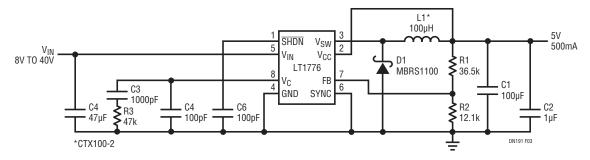
Figure 3. LT1776 Application Circuit for Generating 5V at 500mA
