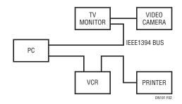
Figure 2. Typical IEEE1394 Bus System Configuration
