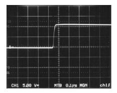
Figure 4. Switch Rise Time at Heavy Loads
