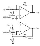
Figure 3. Compensation for Gain < 10
