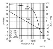
Figure 2. Open-Loop Gain and Phase vs Frequency
