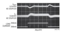
Figure 6. 5V to 12V Boost Converter Transient Response
