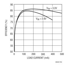
Figure 2. 3.3V to 5V Boost Converter Efficiency
