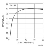
Figure 8. ±15V Dual Output Converter Efficiency
