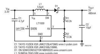
Figure 1. 3.3V to 5V Boost Converter
