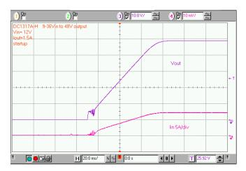
Figure 6. The LT4430 opto coupler driver produces monotonic output voltage rise at startup without output voltage overshoot.
