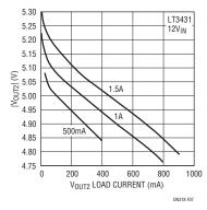
Figure 7. The Negative Supply (V<sub>OUT2</sub>) Maintains ±5% Regulation
