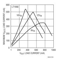
Figure 3. Maximum Load Current Conditions for Figure 1.
