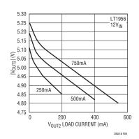
Figure 4. The Negative Supply (V<sub>OUT2</sub>) Maintains ± 5% Regulation
