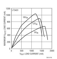
Figure 6. Maximum Load Current Conditions for Figure 2
