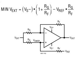
Figure 2. Calculating the Common Mode Input Voltage Range
