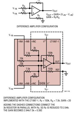
Figure 3. The LT1997-1 Configured as a Difference Amplifier. Gain Is Set by Connecting the Correct Resistors or Combinations of Resistors. Gain of 20 Is Shown, with Dashed Lines Modifying It to a Gain of 0.392
