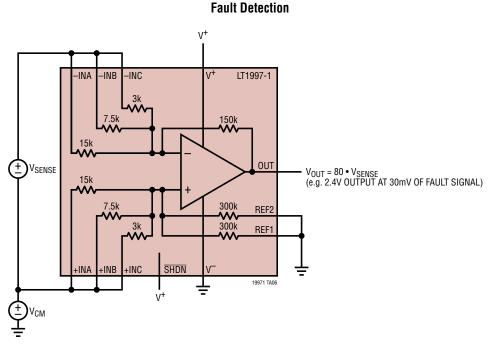
FAULT DETECTION AT HIGH COMMON MODE VOLTAGE: LOOK FOR AN INCREASING VOLTAGE THAT MIGHT INDICATE BREAKAGE.
