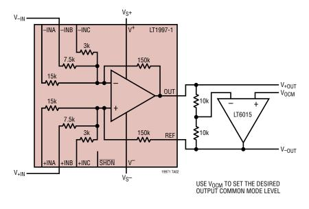
LT1997-1 Configured for Differential Output with Gain = 20
