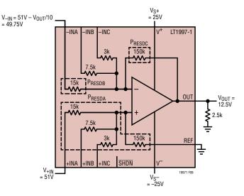
Figure 8. Power Dissipation Example
