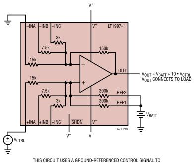
**Create a Supply Using Control Signal**
