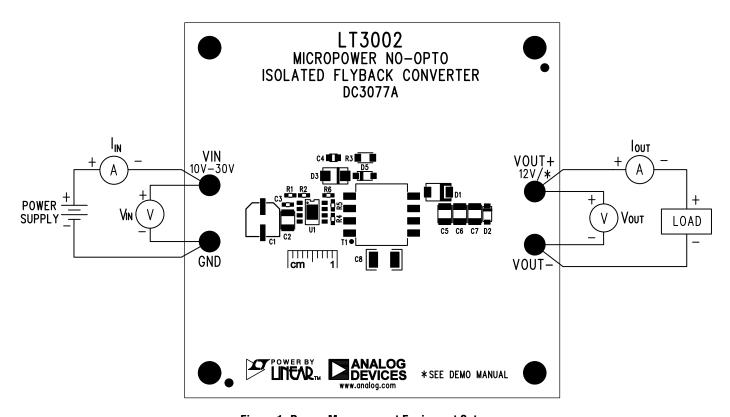
Figure 1. Proper Measurement Equipment Setup
