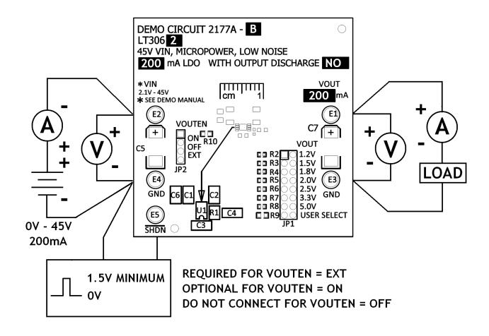
Figure 1: Proper Measurement Equipment Setup for DC2177A-B
