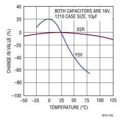
Figure 5. Ceramic Capacitor Temperature Characteristics
