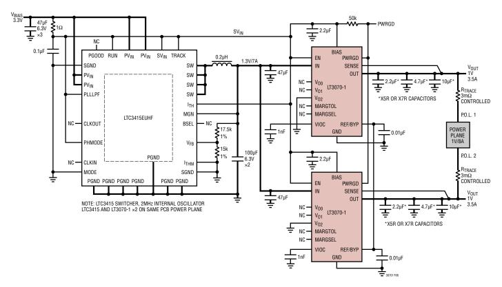
Figure 8. 1V, 7A Point-of-Load Current Sharing Regulators
