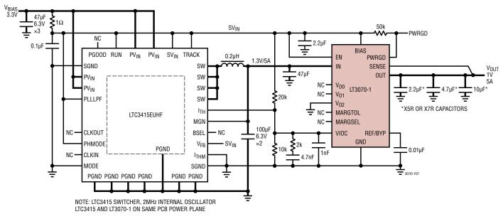
Figure 7. Regulator with VIOC Buck Control
