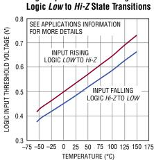
**Logic Input Threshold Voltages**
