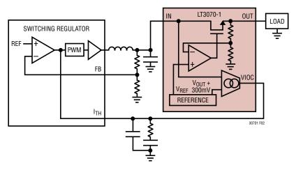
Figure 2. VIOC Control Block Diagram
