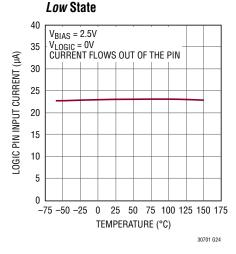
Logic Pin Input Current,
