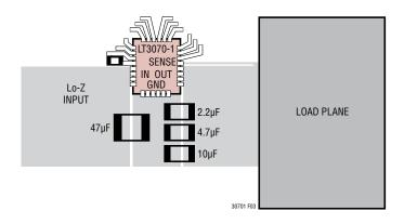
Figure 3. Example PCB Layout
