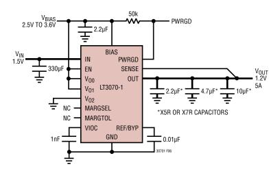
Figure 6. 1.5V to 1.2V Linear Regulator
