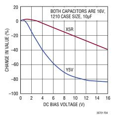
Figure 4. Ceramic Capacitor DC Bias Characteristics
