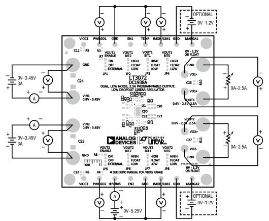
Figure 1. Proper Equipment Setup for DC1938A.
