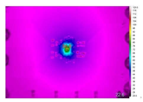
Figure 2. Thermal Image with 3.1V<sub>IN1</sub>, 3.1V<sub>IN2</sub>, 2.5V<sub>OUT1</sub> at 2.5A and 2.5V<sub>OUT2</sub> at 2.5A. Vertical Orientation with No Forced Air.
