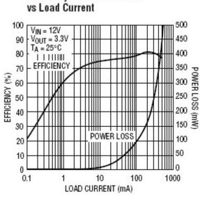
Figure 1. DC1232A Typical Efficiency
