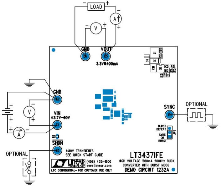
Figure 5. Proper Measurement Equipment Setup
