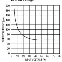
Figure 2. DC1232 Typical Supply Current in Burst Mode
