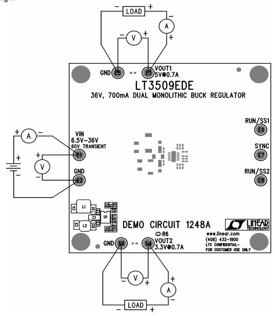
Figure 1. Proper Measurement Equipment Setup
