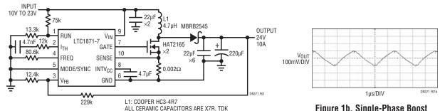
Figure 1a. Single-Phase Boost Converter: Can be Used to Convert 12V Input to 24V, 10A Output
