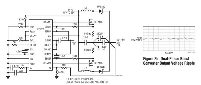
Figure 2a. Dual-Phase Boost Converter Reduces EMI and Ripple Currents with a Minimum Input and Output Filtering
