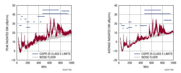
Figure 5. DC2247A Radiated Peak and Average EMI—30MHz to 1GHz—Passes CISPR 25 Class 5 Limits
