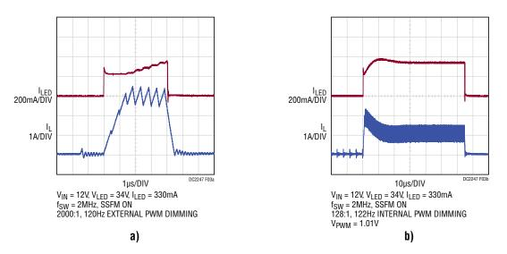
Figure 3. Infinite-Persist Scope Traces Show PWM Dimming and SSFM Working Together for Flicker-Free Brightness Control with both a) Externally and b) Internally Generated PWM Dimming
