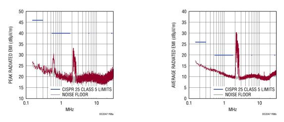
Figure 6. DC2247A Radiated Peak and Average EMI—150kHz to 30MHz—Passes CISPR 25 Class 5 Limits
