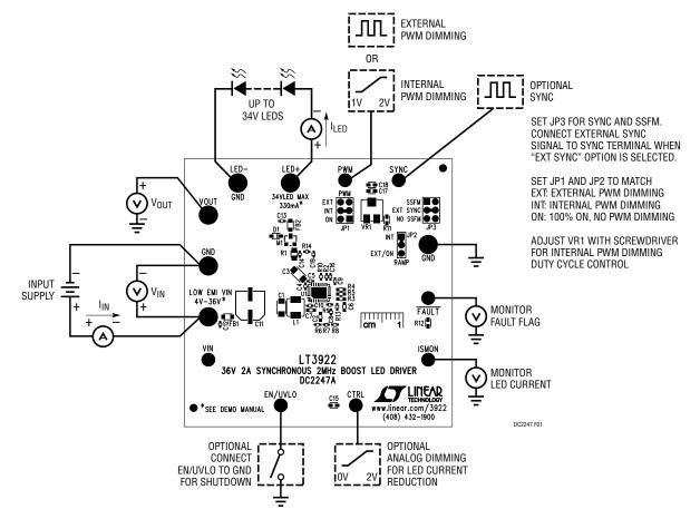
Figure 1. Test Procedure Setup Drawing for DC2247A
