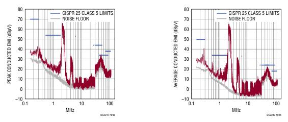
Figure 4. DC2247A Conducted Peak and Average EMI—Passes CISPR 25 Class 5 Limits.
