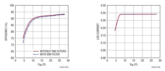
Figure 2. DC2247A Efficiency and LED Current Versus Input Voltage for 34V 330mA LED Load. Efficiency Remains High Through the Range Due to Synchronous Switching. At Low V<sub>IN</sub>, I<sub>LED</sub> Can Be Reduced Due to Peak Switch Current Limit
