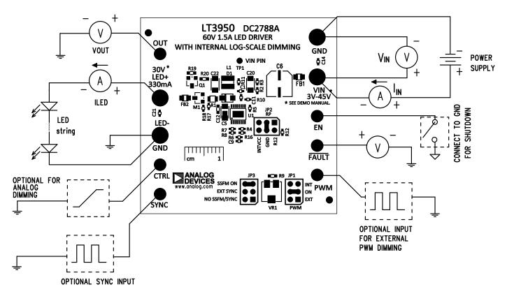
Figure 1. Test Procedure Setup Drawing for DC2788A
