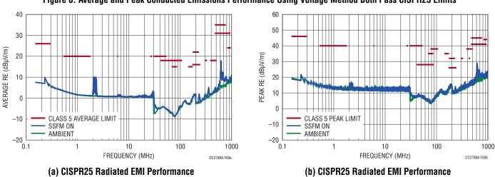
Figure 8. Average and Peak Conducted Emissions Performance Using Voltage Method Both Pass CISPR25 Limits
