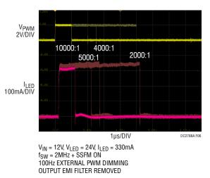
Figure 6. Maximum PWM Dimming Ratio is Very High with Output EMI Filters Removed
