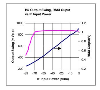
**Figure 2. Baseband I/Q differential output voltage swing and RSSI output versus IF input power.** (IF Frequency = 280MHz, with a 1:4 IF input transformer, and without IF interstage filtering.)
