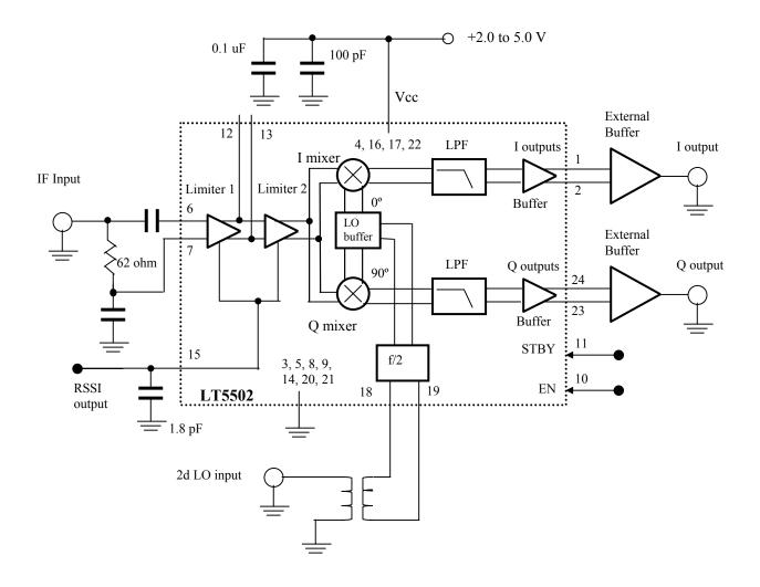
Figure 1. Demo board DC333A block diagram.
