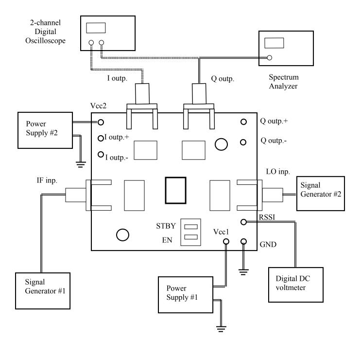
Figure 4. Test and measurement set-up
