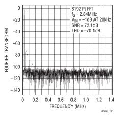
Figure 2. FFT Shows Low Noise and Distortion of Figure 1 Circuit
