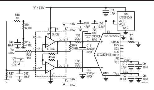
Figure 3. LTC2379-18 Single Supply, ±10V Single-Ended Driver Using the LT6350
