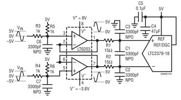
Figure 1. An LTC2379-18 Fully Differential ±5V Driver Using the LT®6203
