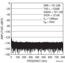
Figure 2. 32k Point FFT Using the Circuit of Figure 1
