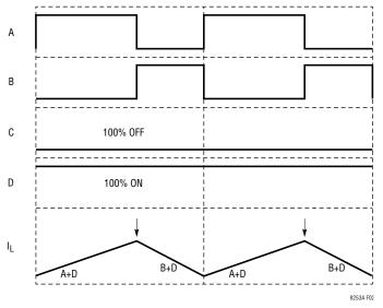
Figure 2. Peak-Buck in Buck Region ( $V_{IN} >> V_{OUT}$ )
