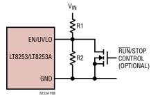
Figure 8. V<sub>IN</sub> Undervoltage Lockout (UVLO)
