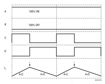
Figure 5. Peak-Boost in Boost Region (V<sub>IN</sub> << V<sub>OUT</sub>)
