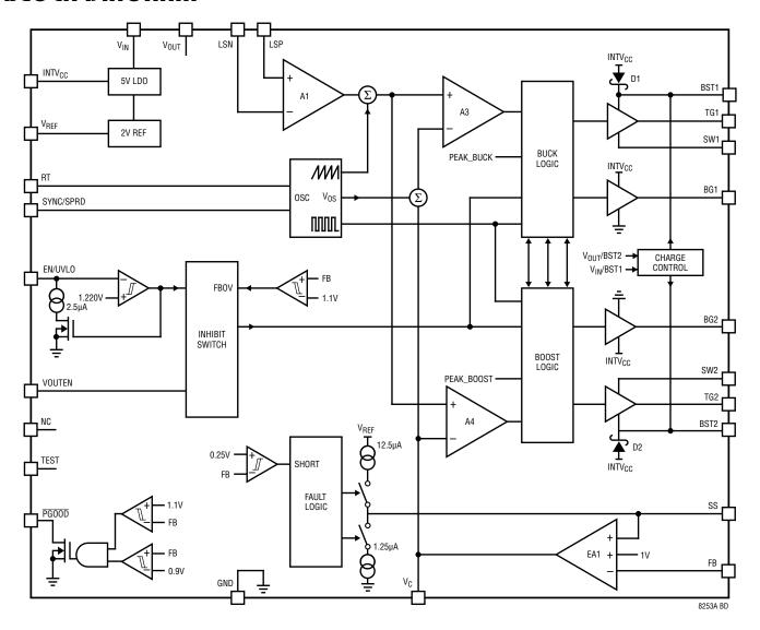
The LT8253/LT8253A are current mode DC/DC controllers that can regulate output voltage from an input voltage above, below, or equal to the output voltage. The proprietary peak-buck peak-boost current mode control scheme uses a single current sense resistor and provides smooth transition between buck region, buck-boost region, and boost region. Its operation is best understood by referring to the Block Diagram.
