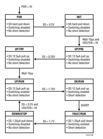
Figure 6. Start-Up and Fault Sequence
