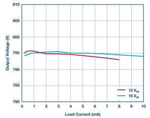
Figure 6. Load regulation of the solution in Figure 4 at various input voltages.
