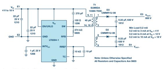
Figure 4. A complete 800 V/10 mA isolated flyback converter from a 4 V to 18 V input.
