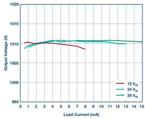
Figure 3. Load regulation of Figure 1 at various input voltages.
