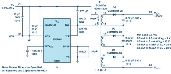
Figure 1. A complete 1000 V/15 mA isolated flyback converter from a 4 V to 28 V input.
