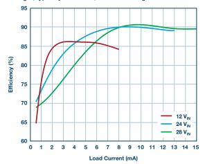
Figure 2. Efficiency of Figure 1 at various input voltages.
